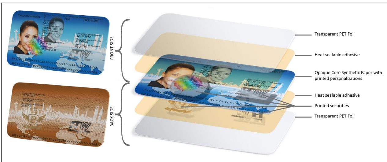
Diagram 9: A typical Teslin®/Synthetic Paper structure
