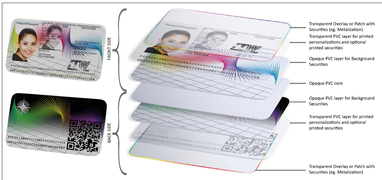
Diagram 1: A typical PVC Card structure with multiple layers
