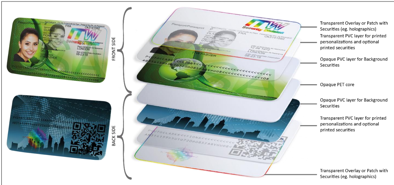
Diagram 2: A typical Composite Card (PVC/PET) structure
