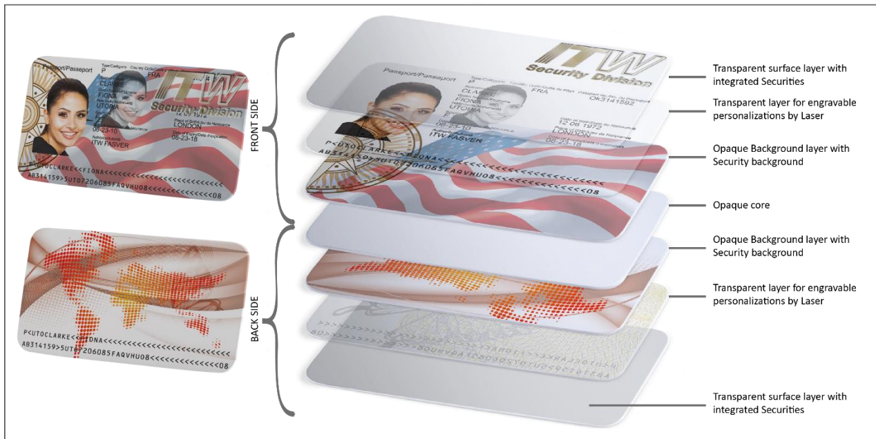
Diagram 4: A typical Polycarbonate Card structure
